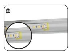
Stick Mylar tape to isolate the cutting position from the bottom of profile inner slot to avoid short-circuit;
