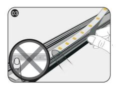
While sticking strips, peel off the release paper of the tape step by step. Don't peel off all release paper at a time to avoid getting your strip in a mess.
