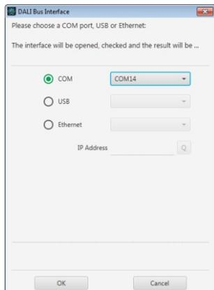
Figure 3: Select Serial Connection Port
