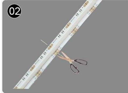
◎ Calculate the needed length and cut off the extra length along cutting mark if necessary; if need to add wires, please weld them at the next location with printed mark.
