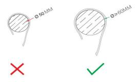
No winding an object with a diameter <5cm</li>
