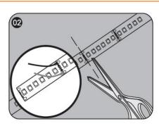
Calculate the needed length and cut off the extra length along cutting mark if necessary; if need to add wires, please weld them at the next location with printed mark.
