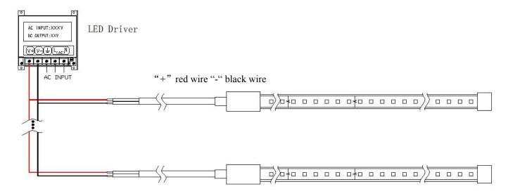
Notes: please make sure the"+"and"-"of the product's input are correctly connected to those of the power supply output.
