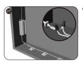
When connect to external power supply, please ensure that the wire's anode & cathode in the first module are connected with the cable of power supply correctly and dispose with waterproof, short-circuit and anti-corrosion.
